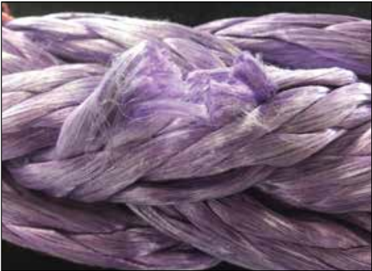
Visual inspection of interior yarns shows one partially cut yarn.
