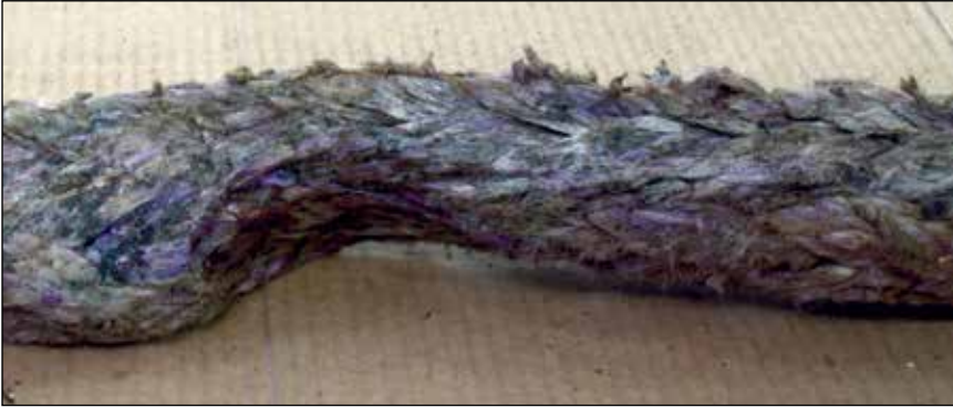
Example of burned and excessively melted fiber
