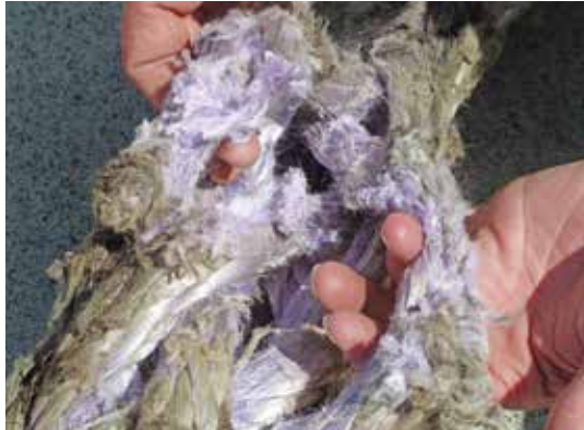
Excessive interior abrasion wear
