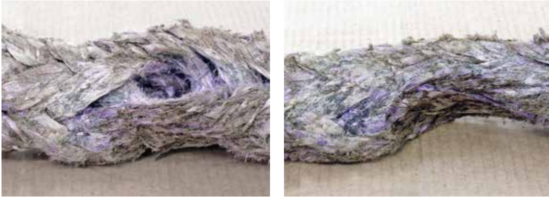
Heat damage on Plasma® rope likely caused by friction heat or slippage. Cover yarns are glazed and fused together. Inspection of the core of the rope on left also shows internal heat. Rope area must cut out or rope retired from service.
