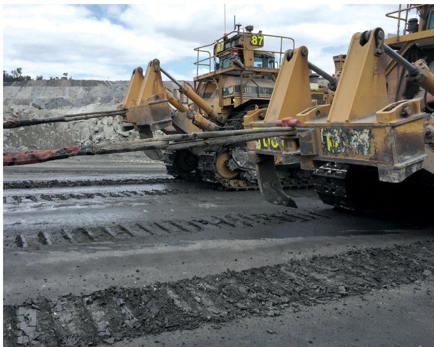
Mining vehicles under tow using Plasma® 12x12 strand ropes
